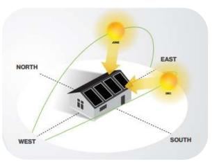
slightly reduced efficiency. Another popular arrangement is to split the panels between the east and west sides of the roof. Although this may require a few additional panels to achieve the same power output, it ensures continuous power generation throughout the day.
