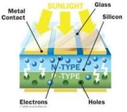
When the photons in the sunlight hit the silicon layers in the PV cells, the electrons are knocked off from the atom. The electric field created by the double silicon layers then
